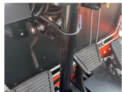
Improved locking mechanism for easy adjustments.
