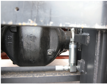
Lift cylinder cushioning for smooth handling.
