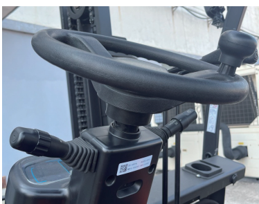
Electro-hydraulic directional switch & multifunction handle (Hydraulic Model) .
