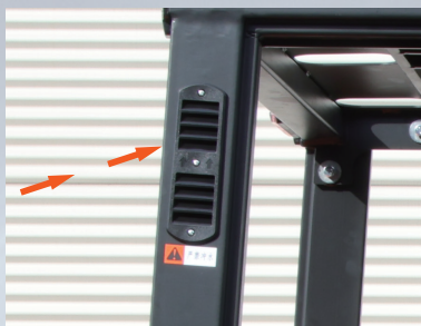
High-position intake grille for optimized airflow.
