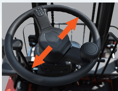
Small-diameter steering wheel for reduced operator effort.
