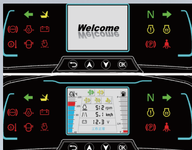
Large LCD display with real-time vehicle status.
